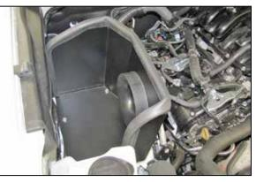
12. Install the heat shield onto the rubber mounted studs installed in the earlier step and secure with the provided hardware.
