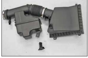
15. Remove the mass air sensor from the factory air filter housing.
