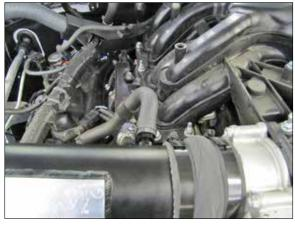
19. Connect the crank case vent fitting onto the vent fitting installed into the K&N<sup>®</sup> intake tube.
