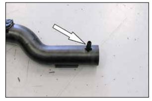
17. Install the provided NPT vent fitting into the  $K\&N^{\ensuremath{\circledast}}$  intake tube as shown.
